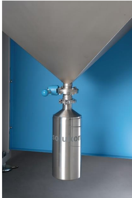
Figure 3: The powder outlet is compatible with standard containers.
