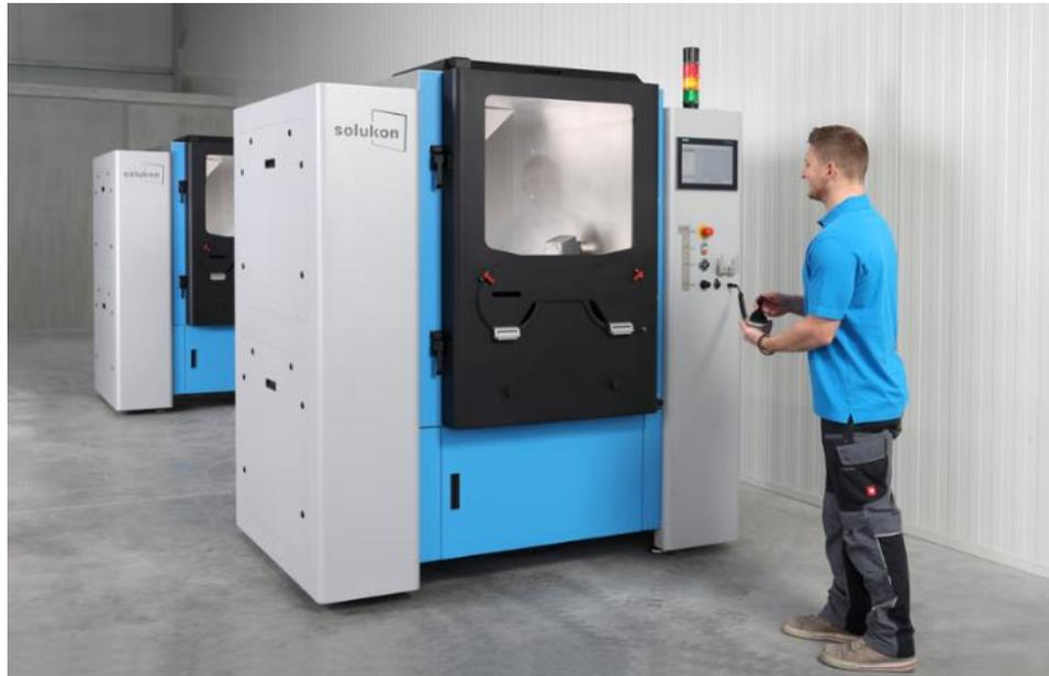
*Figure 1: The new feature, a joystick, here used at SFM-AT-1000-S, enables the operator to move the part in any desired position.*
